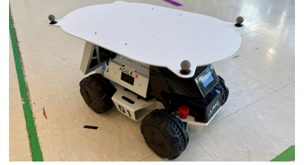
(c). LIMO robot with a landing pad mounted
